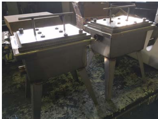
Figure 16. Magnetic traps with holders of the CNano treatment plant.
