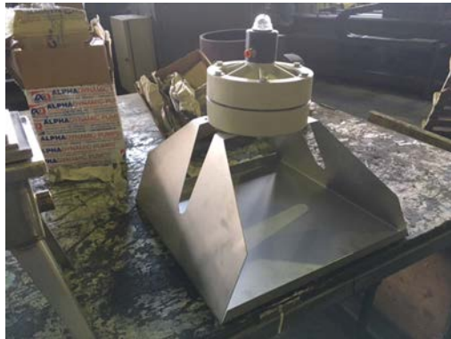
Figure 15. Holder of dampener of the CNano treatment plant.
