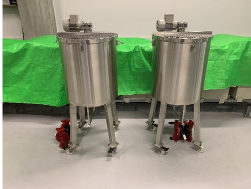
Figure 12. Integrated main reactor systems of the CNano treatment plant.
