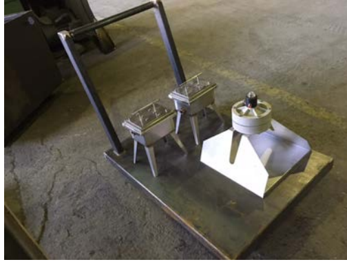
Figure 17. Platform of magnetic traps and pumps of the CNano treatment plant.
