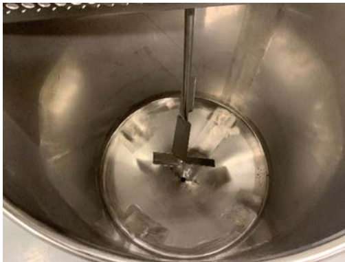
Figure 13. Interior of purification of reactor of the CNano treatment plant.
